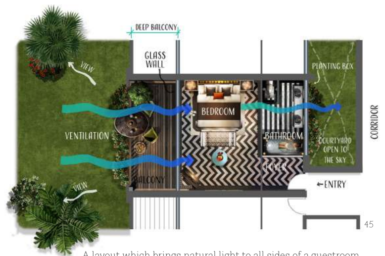
A layout which brings natural light to all sides of a guestroom
