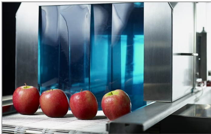
UV light treatment is a non-thermal, non-chemical technology to inactivate microorganisms. Campden BRI's UVI light tunnel can treat products from both above and below.
